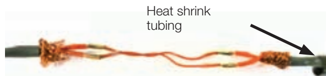
Fig. 3.11 : Push the heat shrink tubing further back and cover with damp cloth before soldering tubes.
