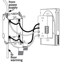
5. Connect the house ground wire to the green or bare lead wire(s) of your floor warming system.
