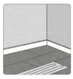
Before fitting the floor covering switch on the heating mat to check that it is working - warmth should be noticeable on the surface of the heating mat within minutes.
