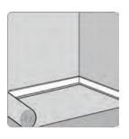
To prevent damage to the mats, special attention should be given to ensure that no nails, screws, staple, tacks are protruding from the sub floor before the underlayment/insulation is installed.
