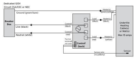
NOTE: All electrical work must be performed by a qualified electrician in accordance with local building & electrical codes and The Canadian Electrical Code, part 1 in Canada or the National Electrical Code in the USA, especially Article 424, Part V of the NEC ANSIINFPA 70.
